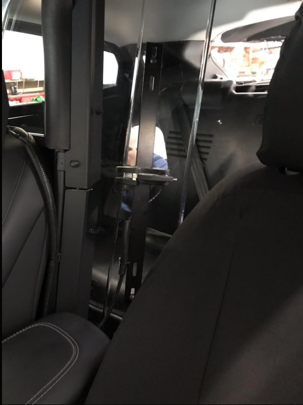
SC-917-5 utilizing the SC-503 24" slide rail for rapid adjustments pictured.
