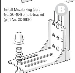
Mark screw locations on wall/floor.Check back side of wall for fuel or electric lines.
