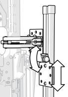
Parts of the weapon may interfere with parts of Mounting Hinge (No. SC-9302). In this case turn the hinge around 180 degrees.
