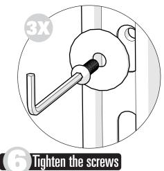
Place your weapon in the setup, test and retest your installation by repeatedly inserting and removing the weapon from the assembly. When satisfied, tighten all screws and test again.
