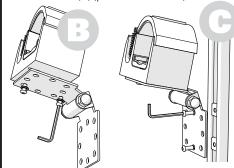
Use 2 x Universal Rail Nuts (part No. SC-5301) and 2 x Allen Head Bolts (part No. SC-8002)
