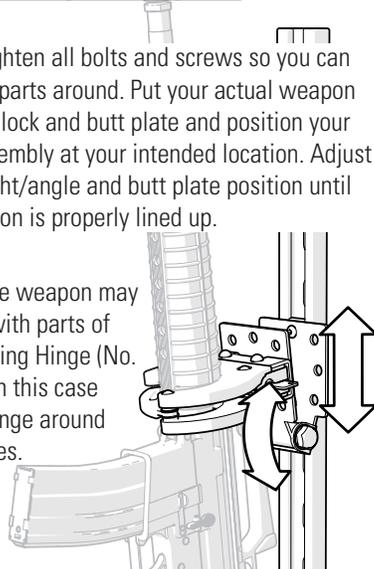
Warning: If you close the ratchet arm tightly on your firearm, you will have to press or tap the outer rubber surface of the ratchet arm when deploying the firearm. This will release the backup safety inside the gun lock, releasing your weapon.
