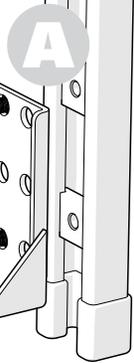
Install Butt Plate (No. SC-1900) on L-bracket (part No. SC-9903) as illustrated, using allen screws and metal screws provided with the butt plate.
