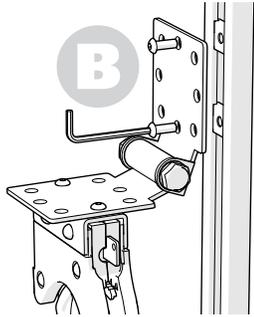
Use 2 x Universal Rail Nuts (part No. SC-5301) and 2 x Allen Head Bolts (part No. Sc-8002)
